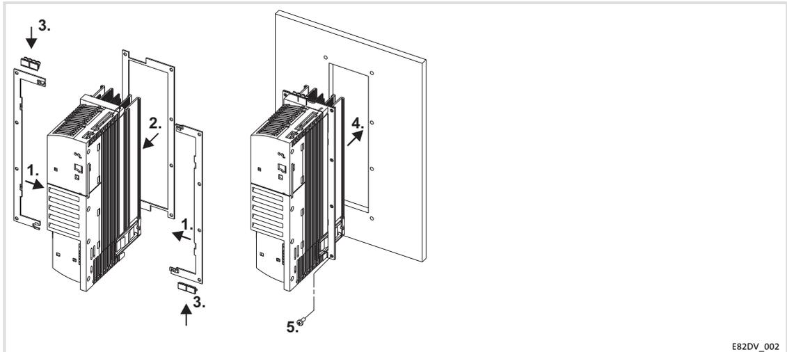
Fig. 5-5 Thermally separated mounting 1.5 ... 2.2 kW
