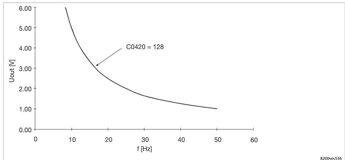
Fig. 10-15 Output signal of the function "1/output frequency"
