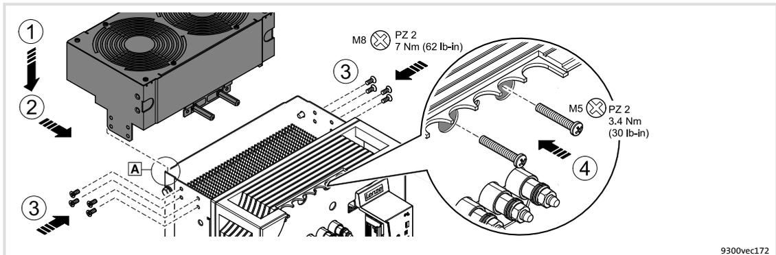
Fig. 5-29 Mounting the fan module on the controller
