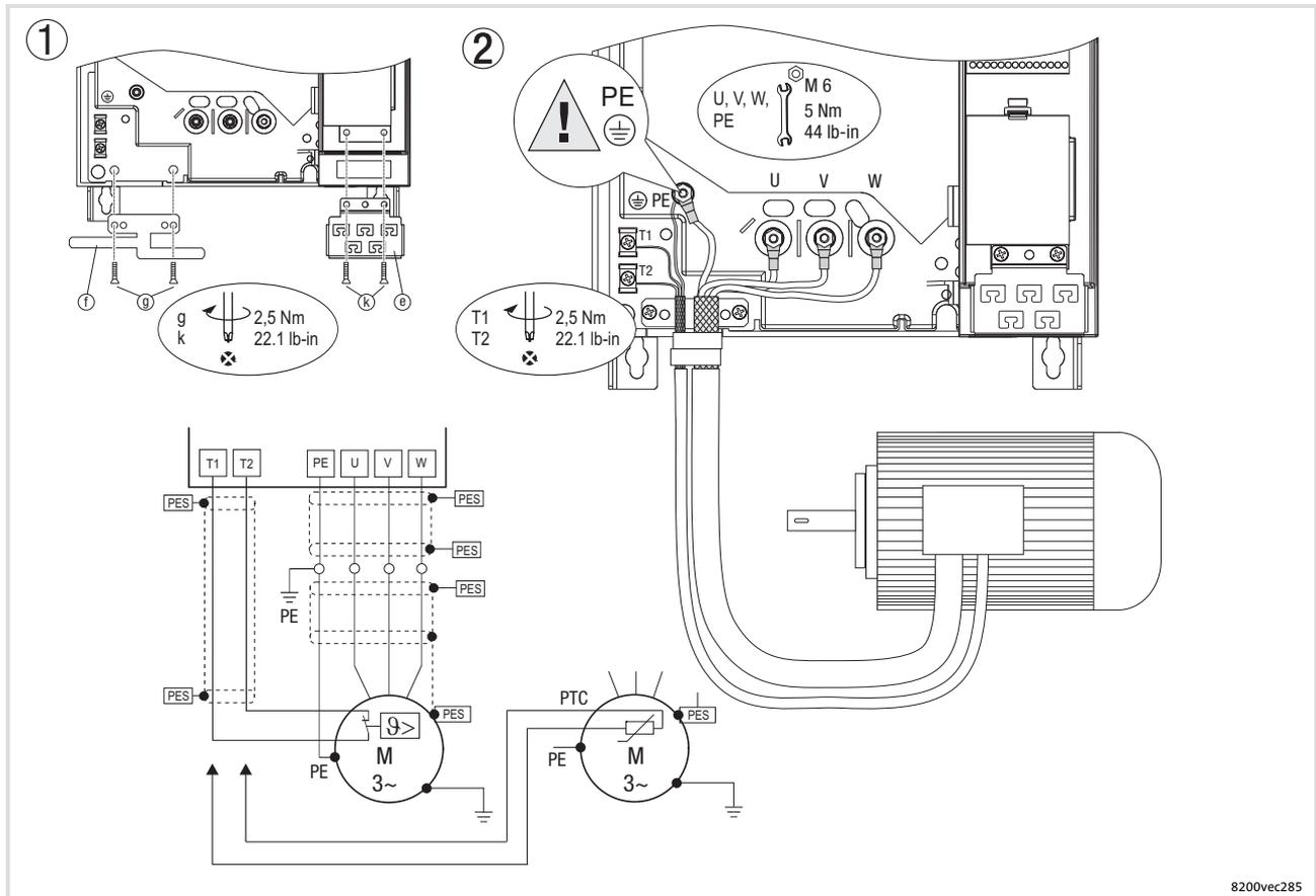
Fig. 6-19 Motor connection 15 ... 30 kW
