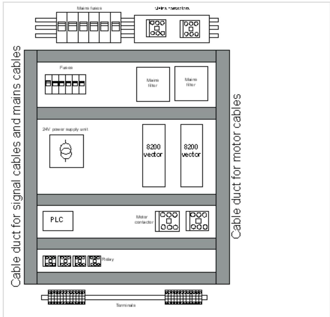
Fig. 6-5 Cable routing in the control cabinet
