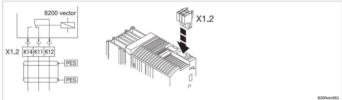
Fig. 6-16 Relay connection 3 ... 11 kW
