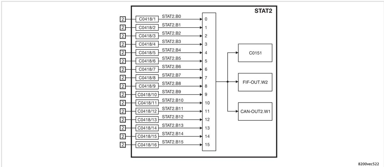
Fig. 16-19 Signal flow in the STAT2 controller state
