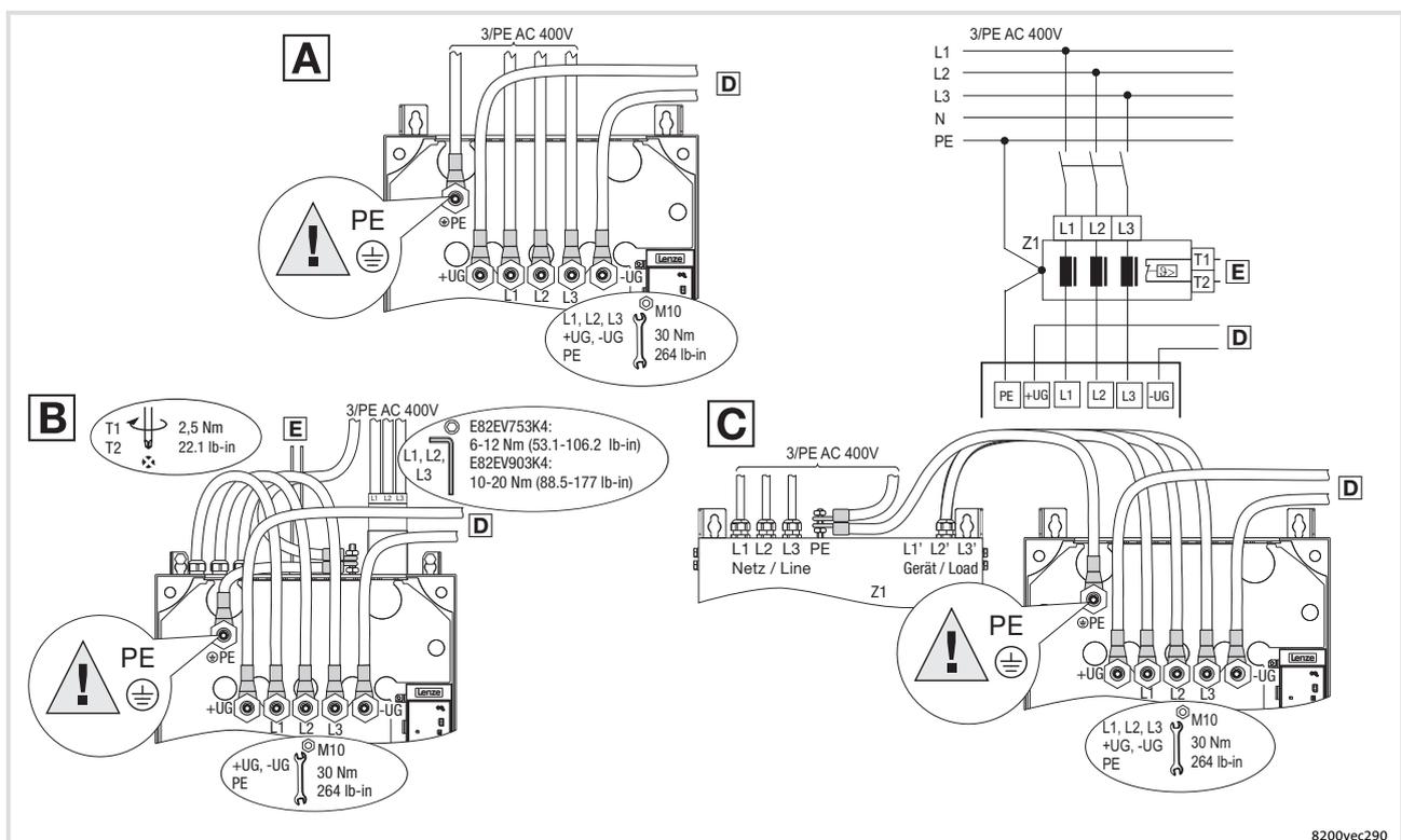
Fig. 6-26 Mains connection 75 ... 90 kW
