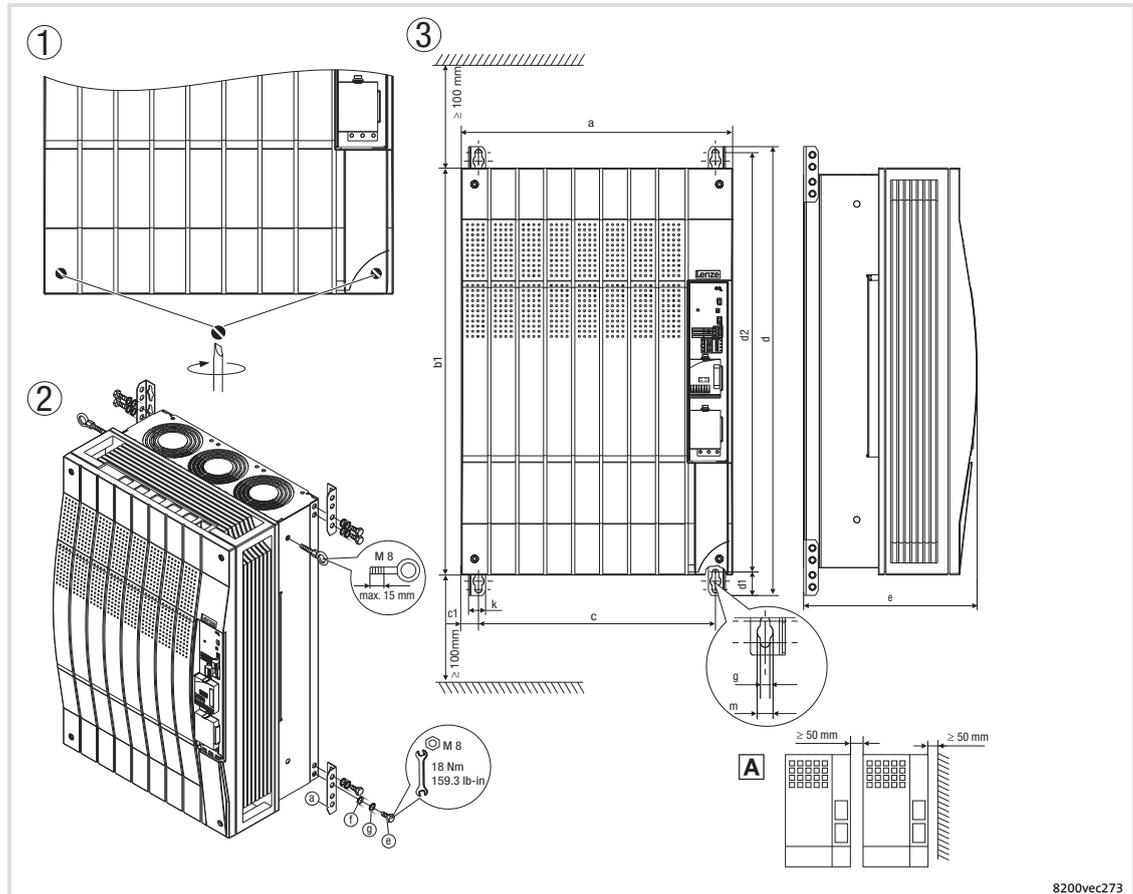
Fig. 5-30 Standard mounting with fixing brackets 75 ... 90 kW
