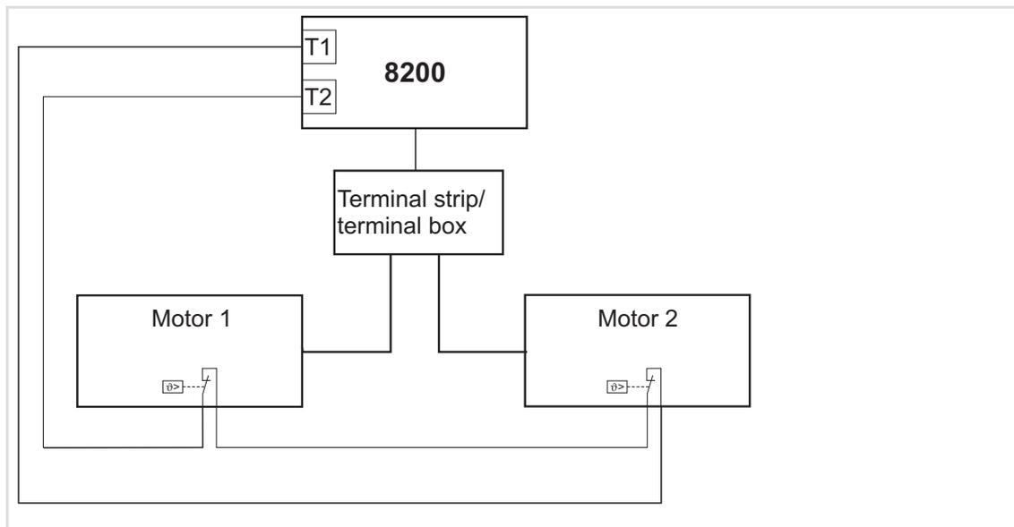
Fig. 15-4 Basic structure of a group drive
