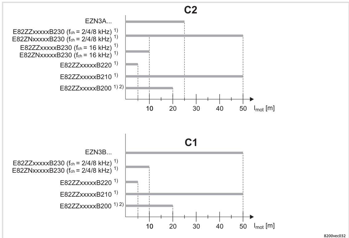
Fig. 6-2 Permissible motor cable lengths<sup>1)</sup> depending on the filter type for compliance with limit class C2 or C1
