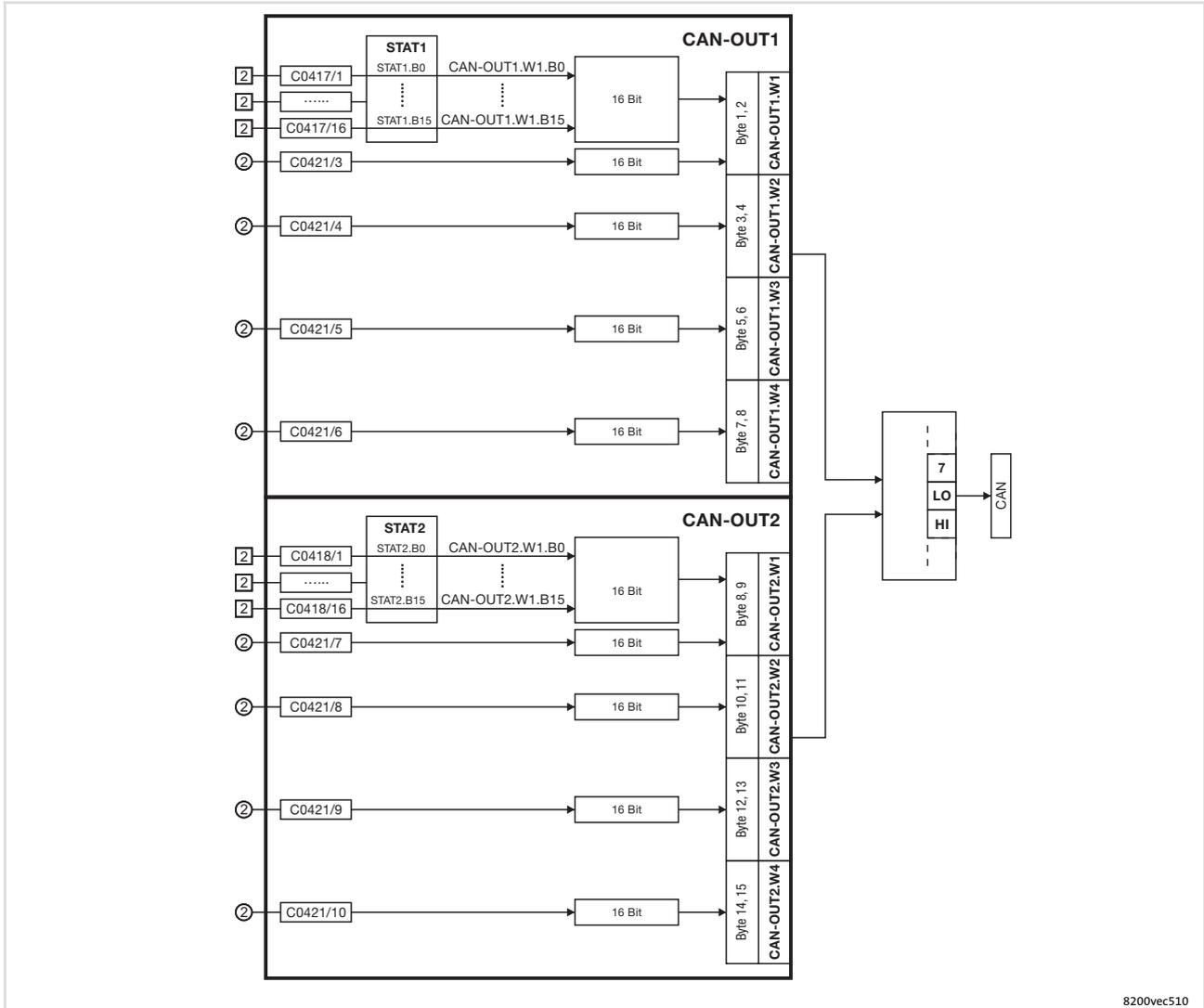
Fig. 16-21 Signal flow in CAN objects CAN-OUT1 and CAN-OUT2
