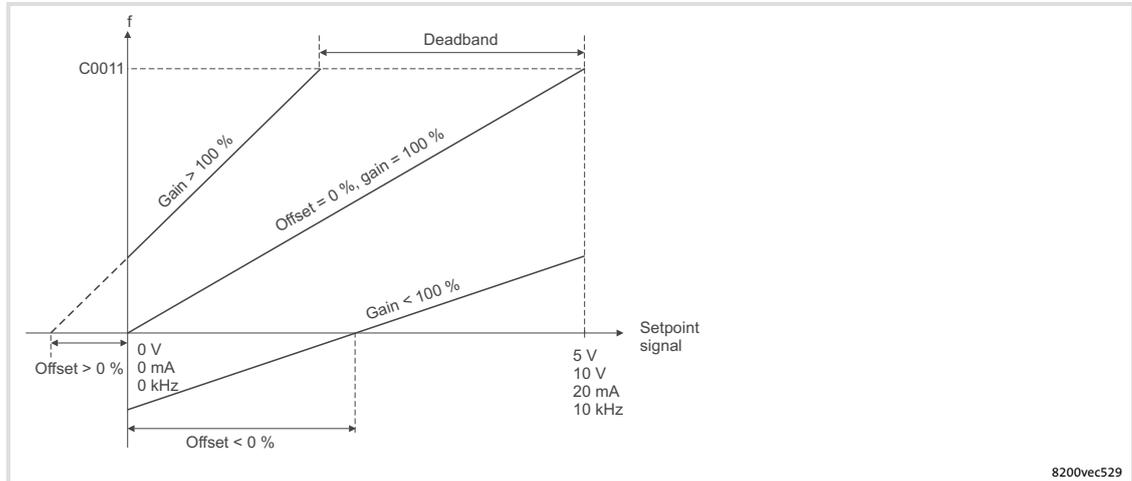
Fig. 10-8 Gain and offset at unipolar setpoint selection
