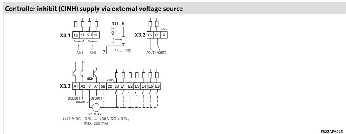
Minimum wiring required for operation
