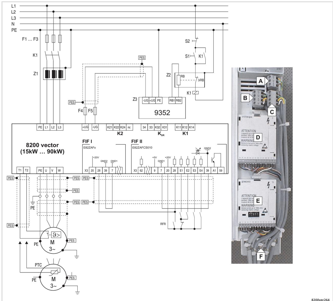
Fig. 6-17 Wiring according to EMC requirements 15 ... 90 kW
