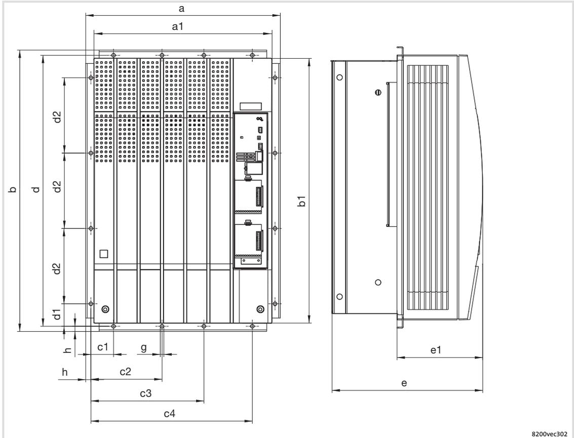
Fig. 5-22 Dimensions for thermally separated mounting 45 kW
