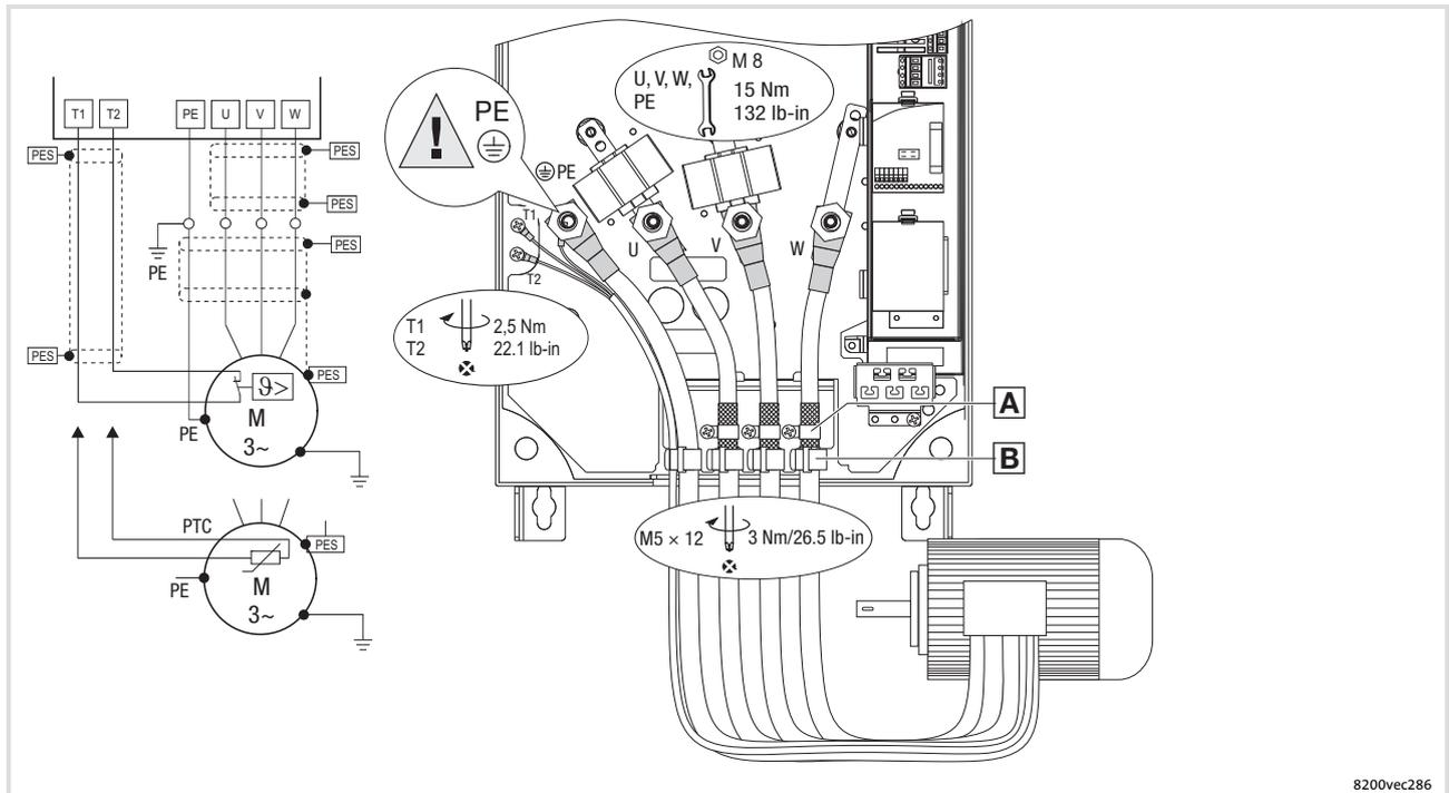
Fig. 6-23 Motor connection 45 ... 55 kW
