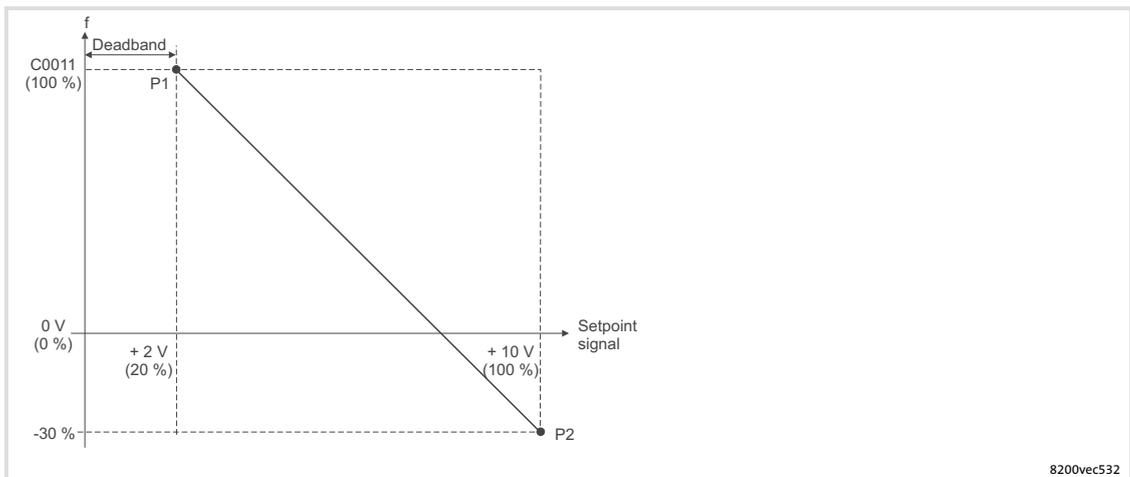
Fig. 10-11 Calculation example for gain and offset
