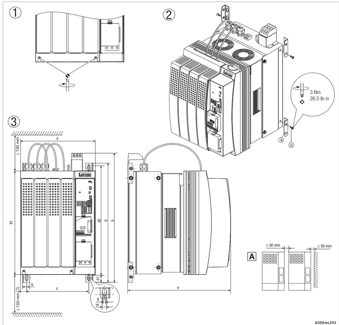
Fig. 5-17 Standard installation with fixing bracket 15 ... 30 kW
