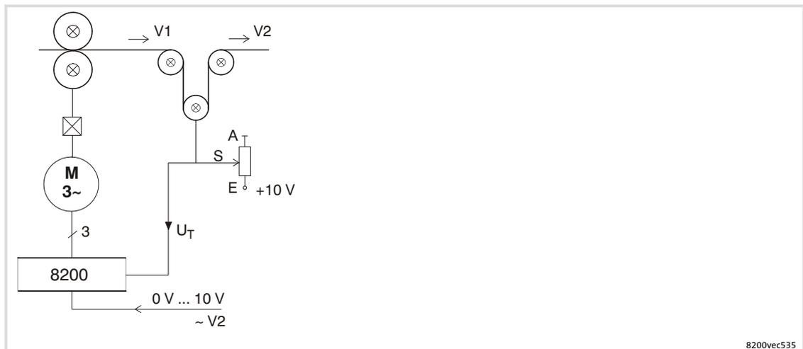
Fig. 10-14 Example: Dancer control with subtractive influence of the process controller
