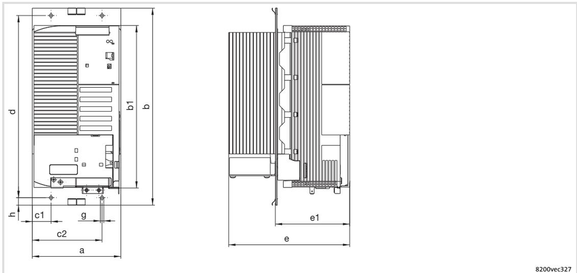
Fig. 5-11 Dimensions for thermally separated mounting 3 ... 11 kW
