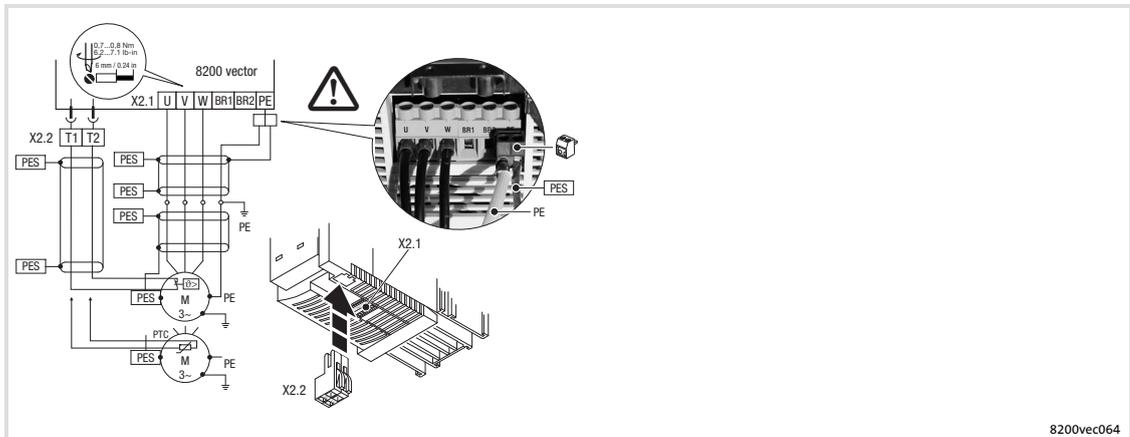
Fig. 6-15 Motor connection 3 ... 11 kW
