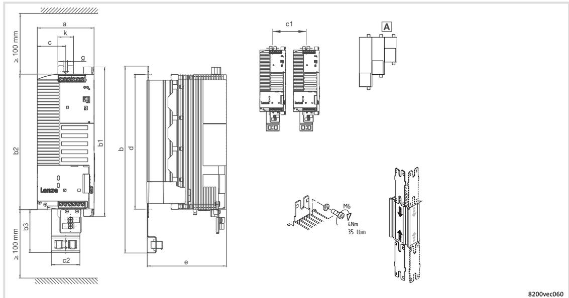
Fig. 5-10 Standard installation with fixing rails 3 ... 11 kW
