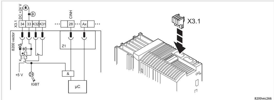
Fig. 14-2 Connection of safety relay K<sub>SR</sub>
