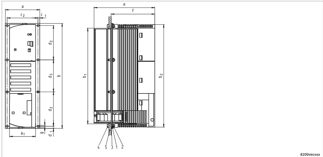
Fig. 5-4 Dimensions for thermally separated mounting 1.5 ... 2.2 kW
