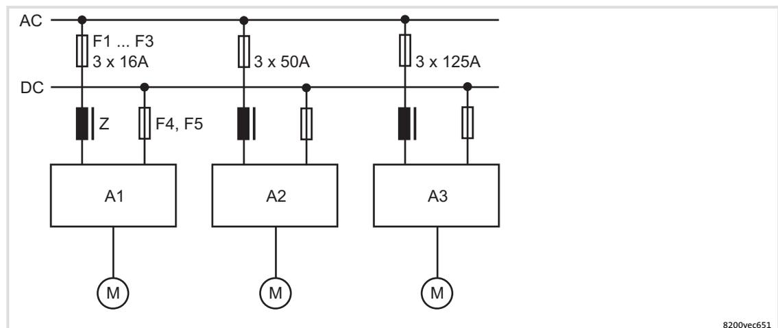
Fig. 12-2 Example: DC connection of three controllers
