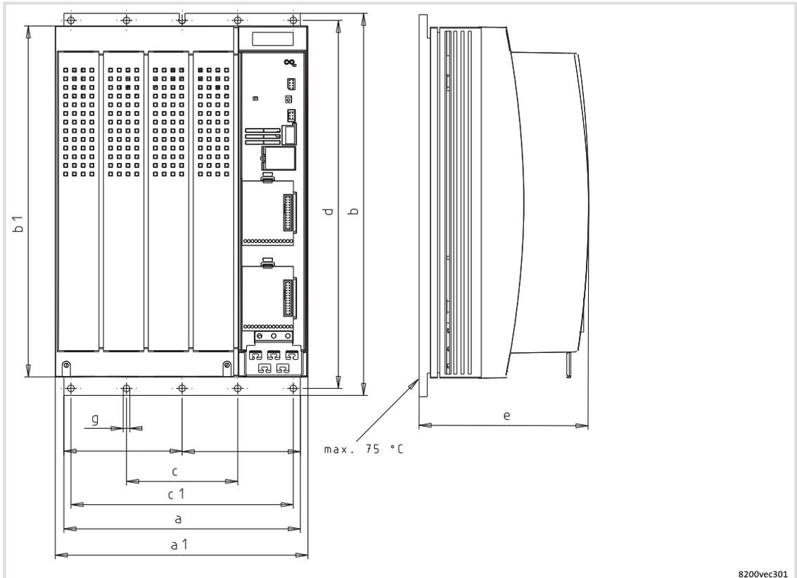
Fig. 5-19 Dimensions for installation in "cold-plate design" 15 ... 22 kW
