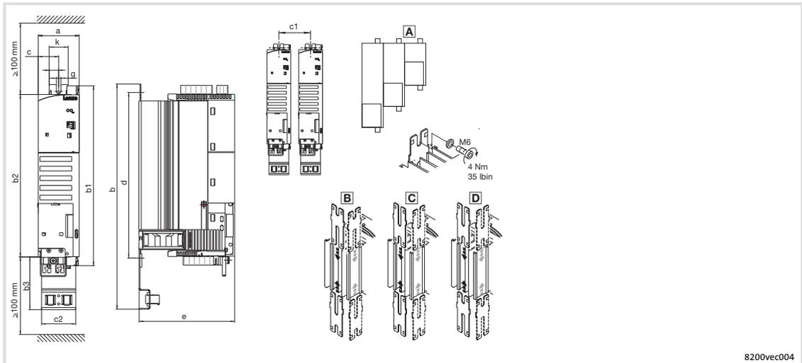
Fig. 5-1 Standard installation with fixing rails 0.25 ... 2.2 kW
