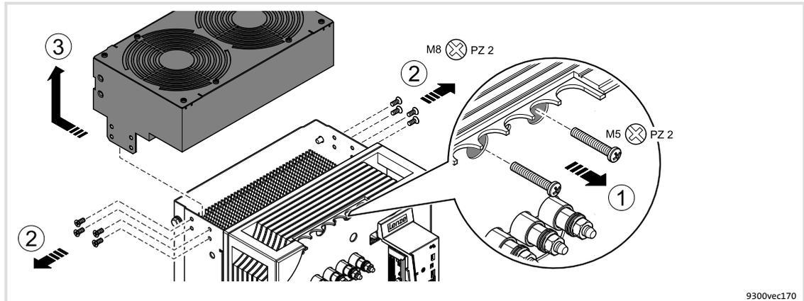
Fig. 5-26 Removing the fan module from the controller
