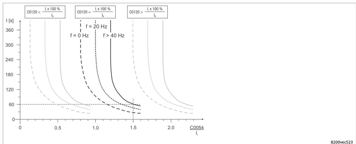
Fig. 10-16 Tripping characteristic of I<sup>2</sup>t monitoring
