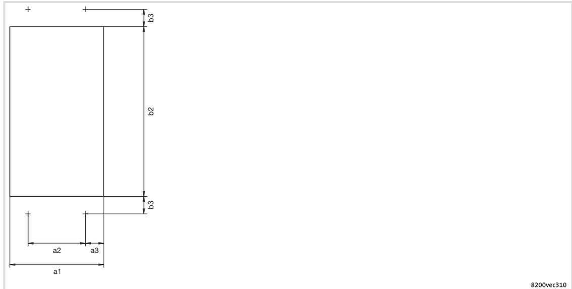
Fig. 5-12 Dimensions for thermally separated mounting cutout 3 ... 11 kW
