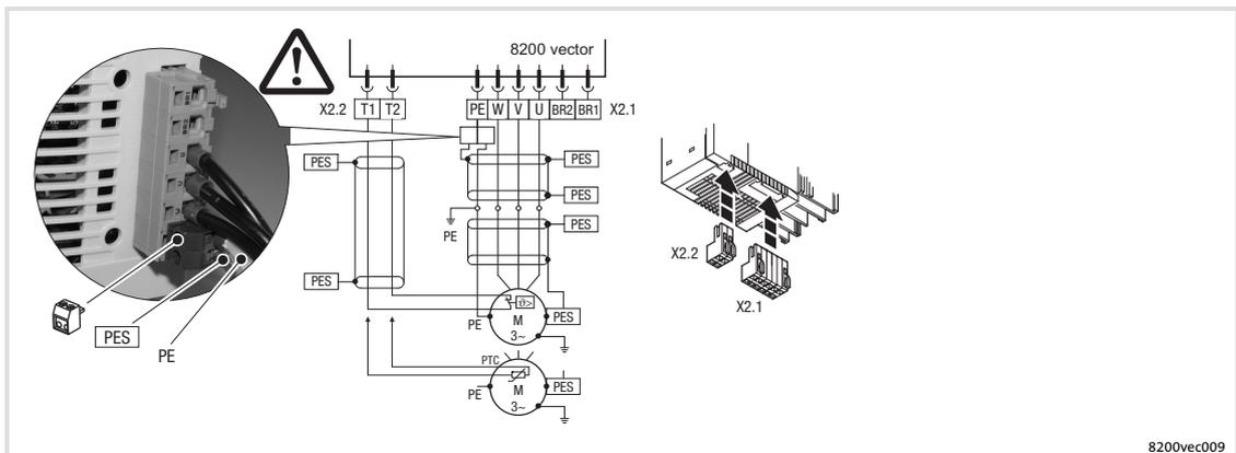
Fig. 6-10 Motor connection 0.25 ... 2.2 kW
