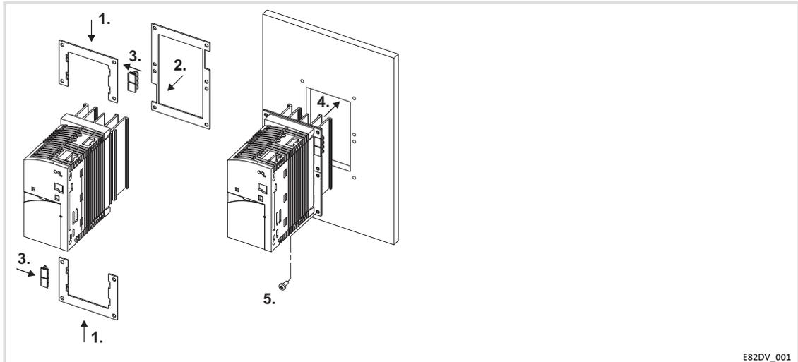
Fig. 5-3 Thermally separated mounting 0.25 ... 0.75 kW
