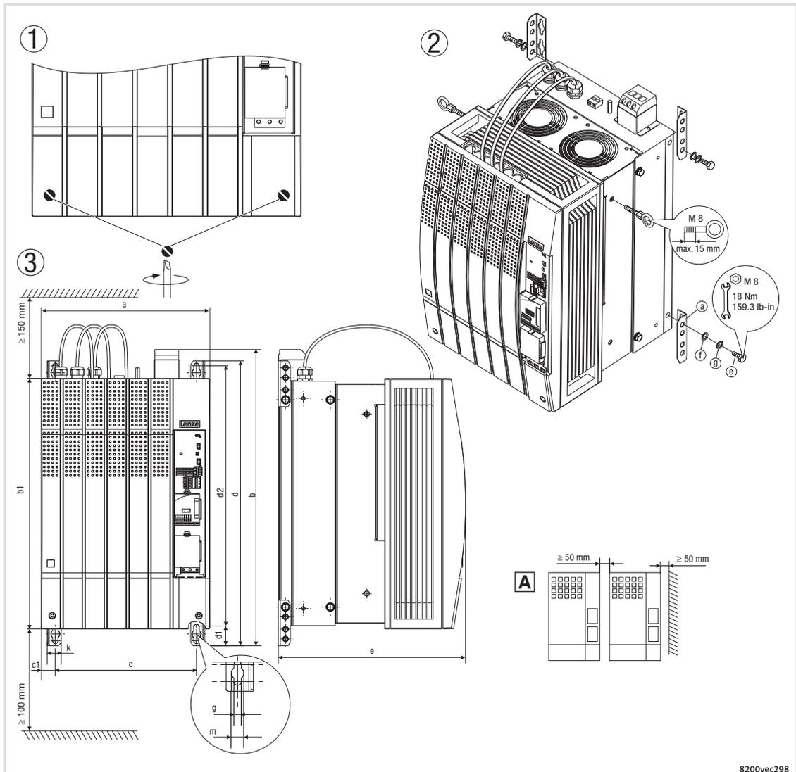
Fig. 5-21 Standard mounting with fixing brackets 45 kW
