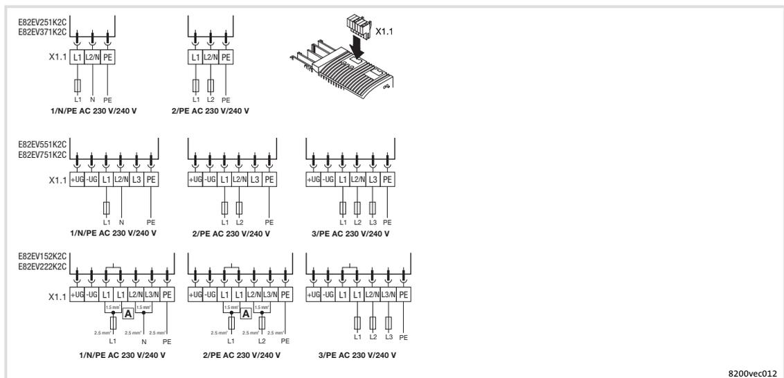
Fig. 6-8 Mains connection 230/240 V 0.25 ... 2.2 kW
