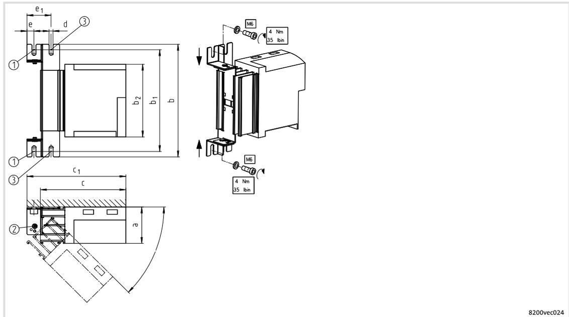
Fig. 5-15 Swivelling lateral mounting
