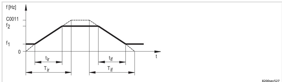
Fig. 10-6 Acceleration times and deceleration times for linear ramp function generator
