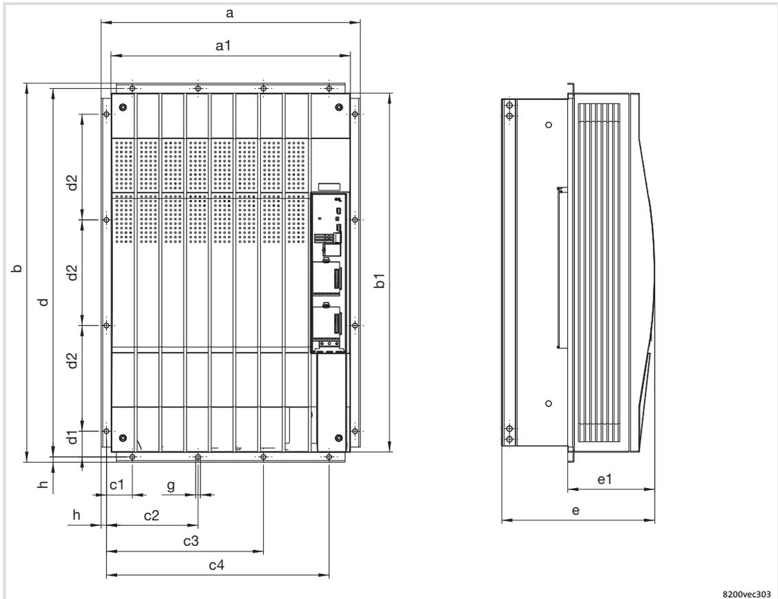
Fig. 5-32 Dimensions for thermally separated mounting 75 ... 90 kW
