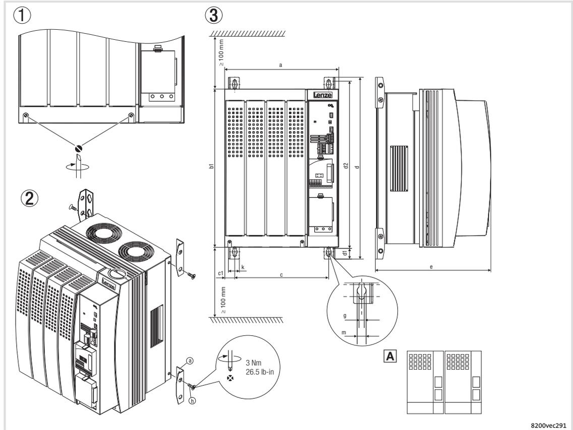
Fig. 5-16 Standard installation with fixing bracket 15 ... 30 kW
