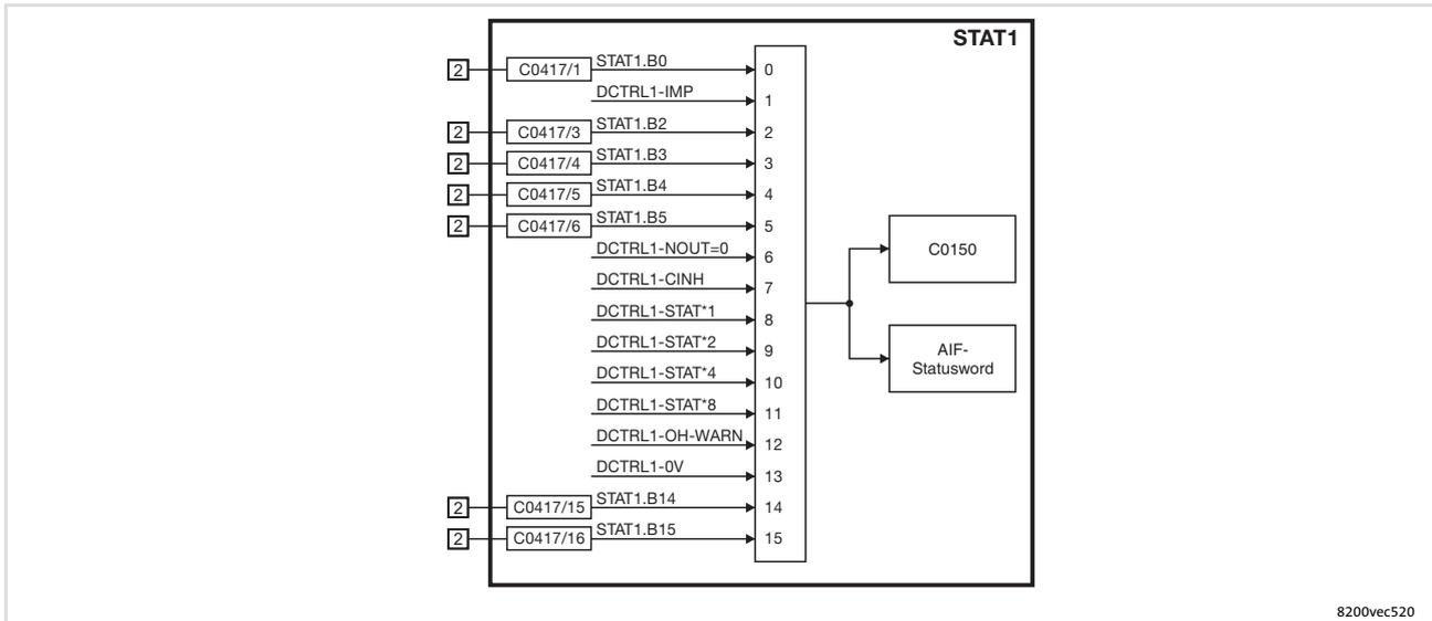
Fig. 16-17 Signal flow in the STAT1 controller state
