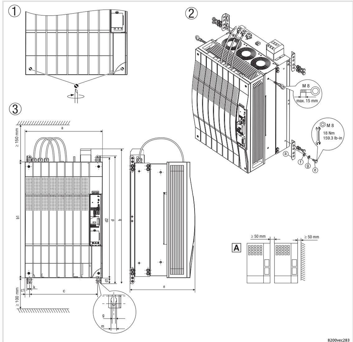
Fig. 5-31 Standard mounting with fixing brackets 75 ... 90 kW
