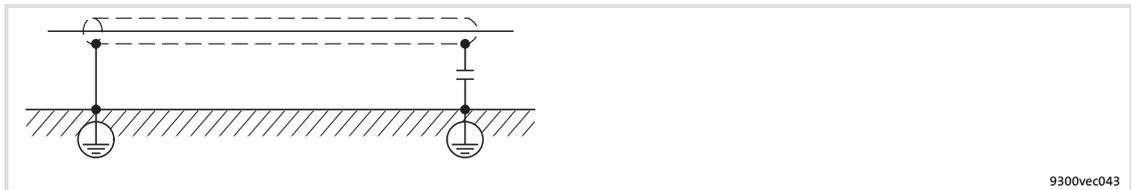
Fig. 6-4 Shielding of long, analog control cables
