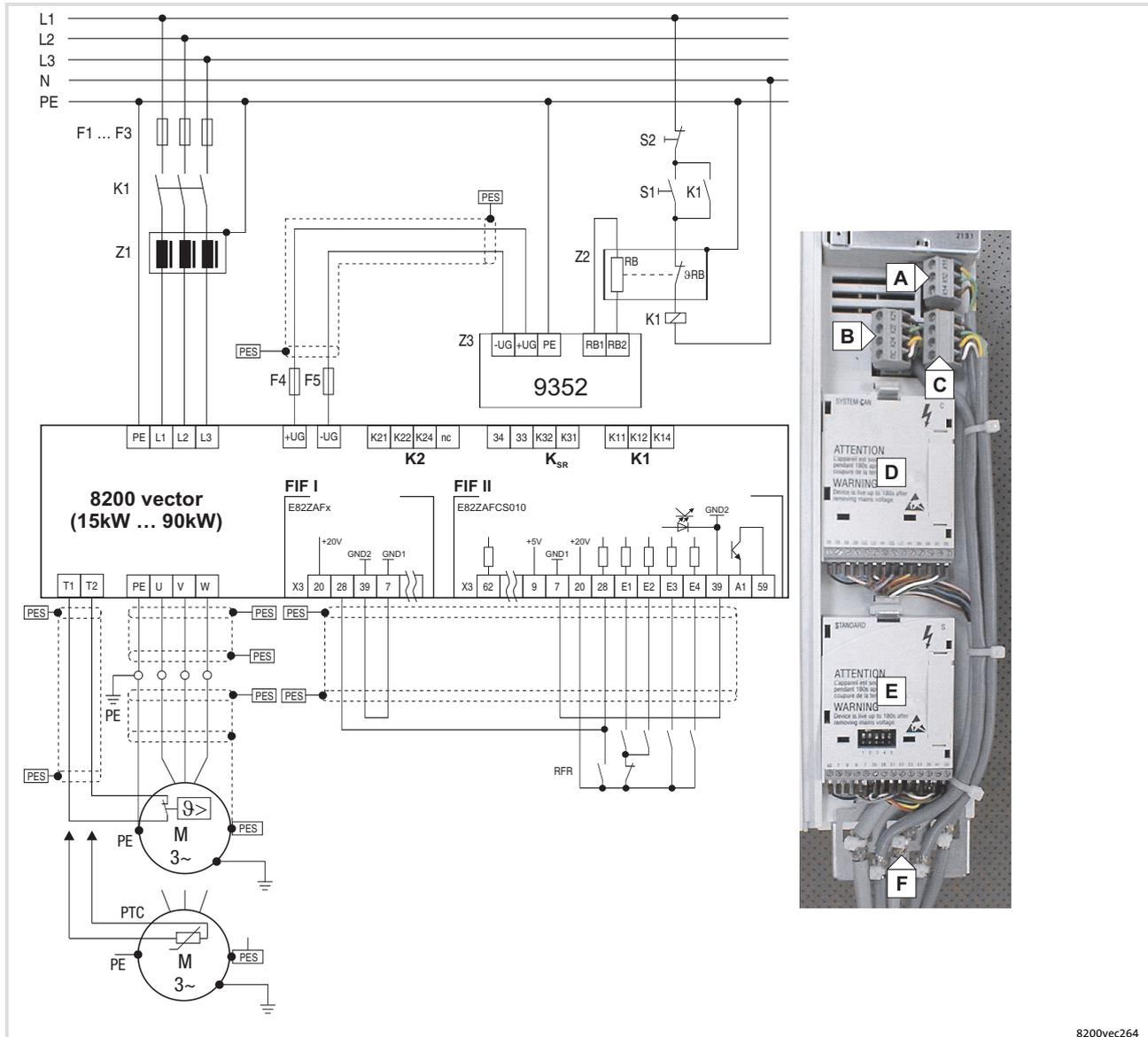
Fig. 6-25 Wiring according to EMC requirements 15 ... 90 kW
