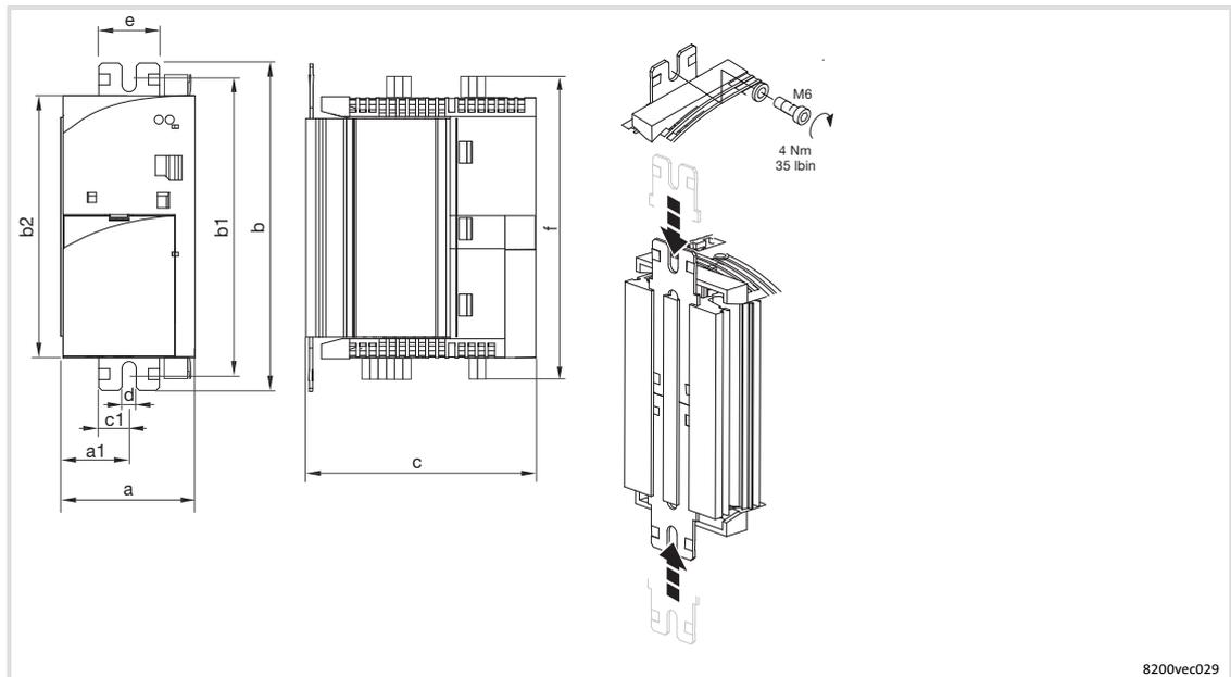
Fig. 5-6 Dimensions for installation in "cold-plate design" 0.25 ... 2.2 kW
