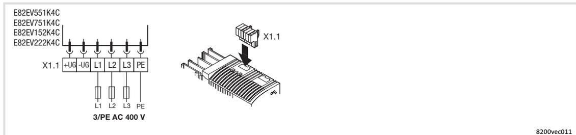
Fig. 6-9 Mains connection 400/500 V 0.55 ... 2.2 kW
