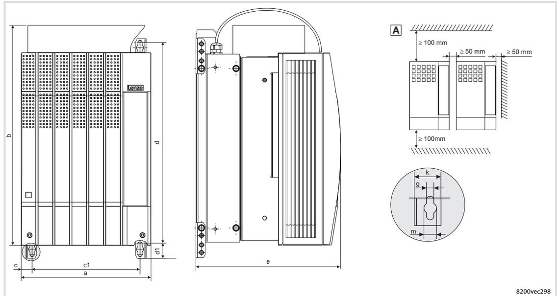
Fig. 5-24 Standard mounting with fixing brackets 55 kW
