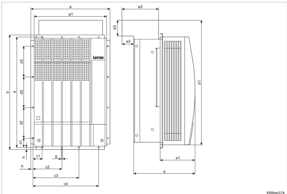
Fig. 5-25 Dimensions for thermally separated mounting 55 kW
