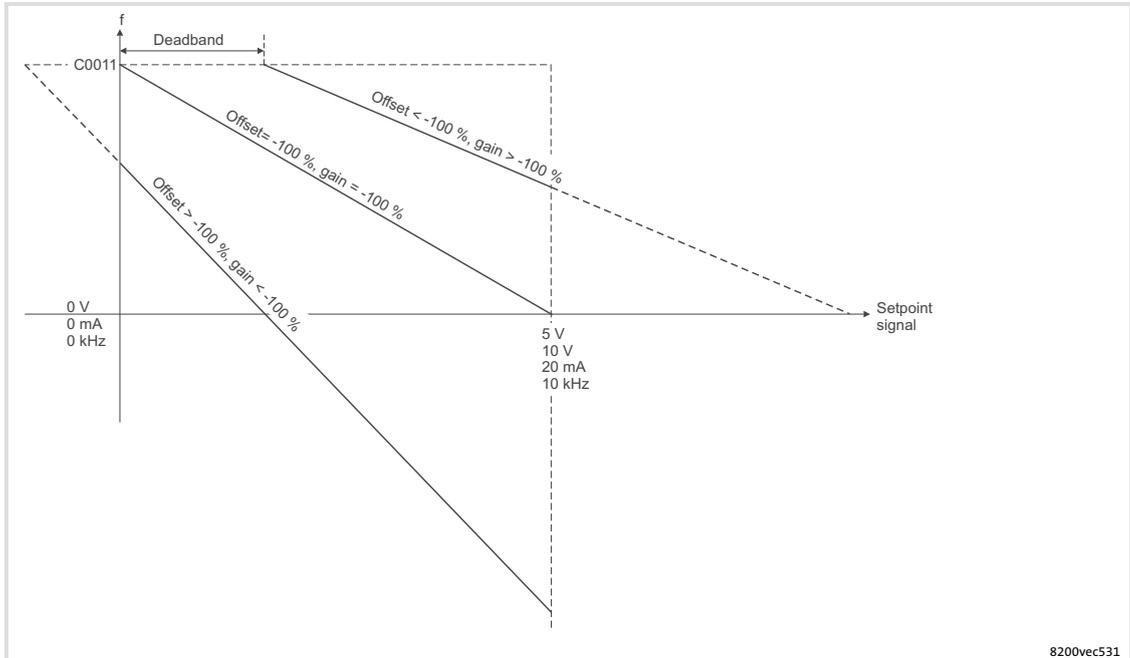
Fig. 10-10 Gain and offset at inverse setpoint selection
