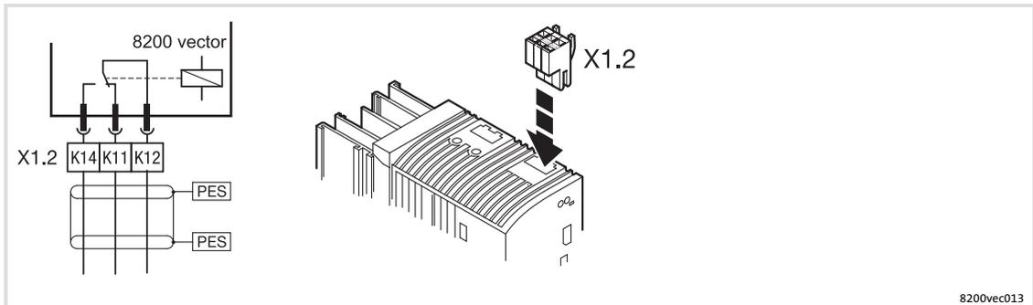
Fig. 6-11 Relay connection 0.25 ... 11 kW
