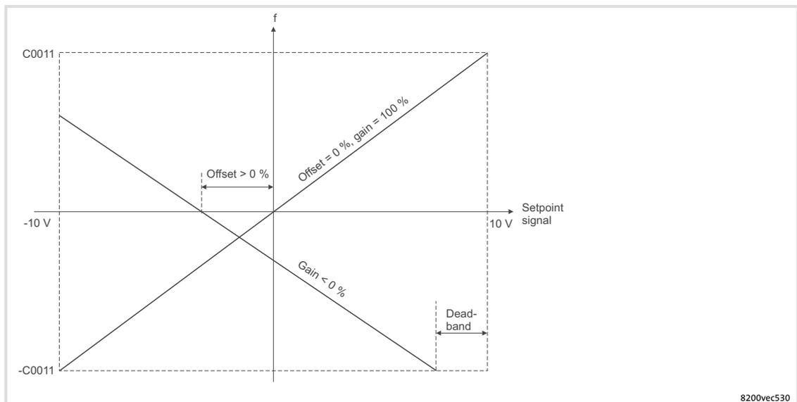
Fig. 10-9 Gain and offset at bipolar setpoint selection
