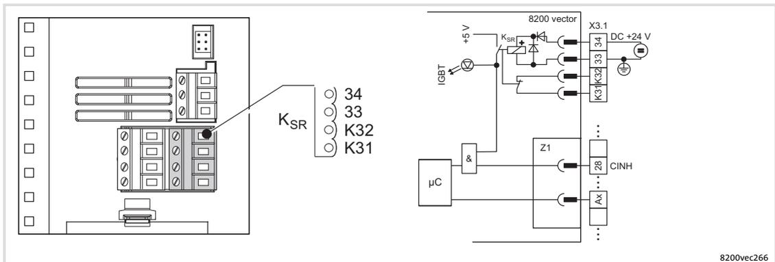
Fig. 14-3 Connection of safety relay K<sub>SR</sub>
