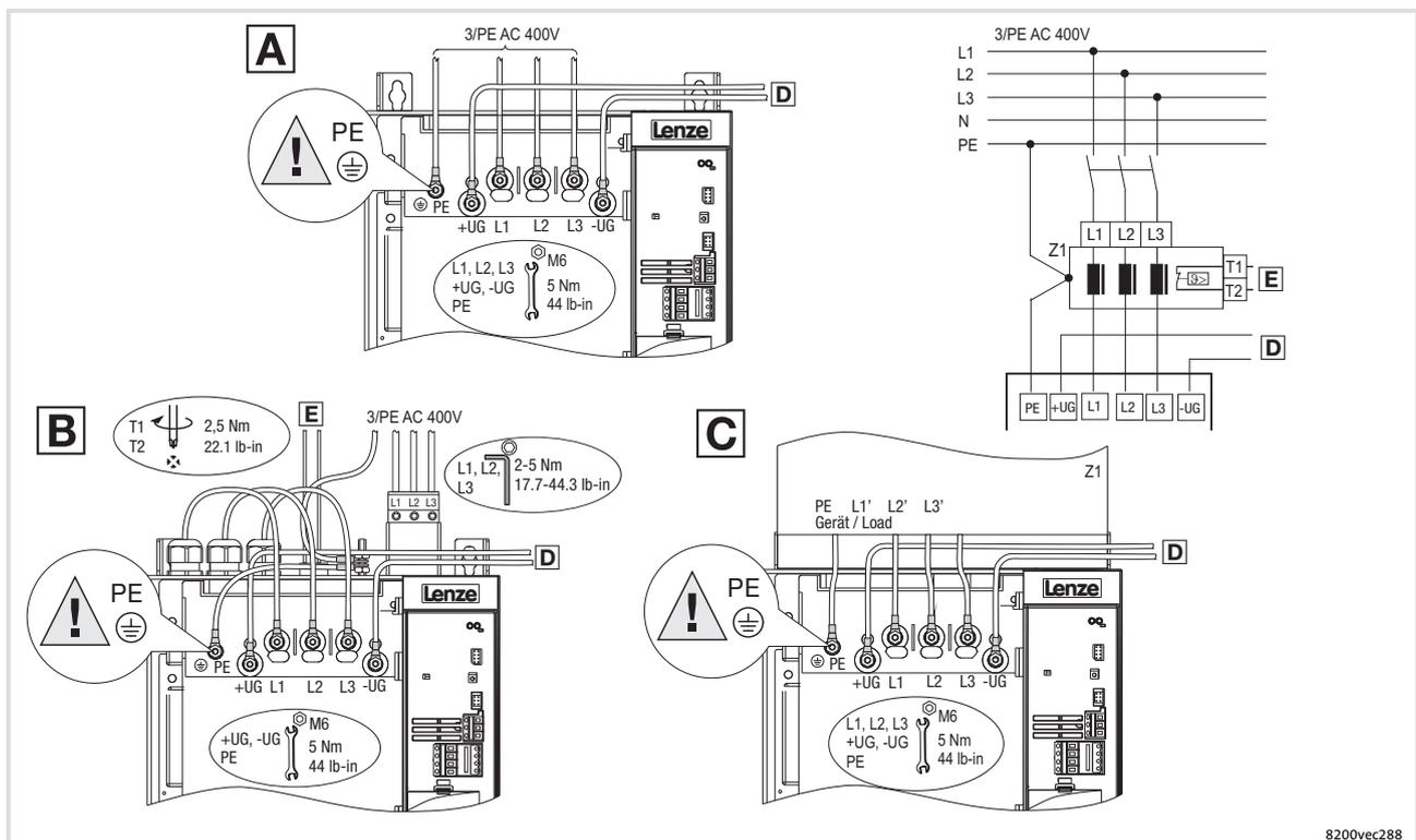
Fig. 6-18 Mains connection 15 ... 30 kW
