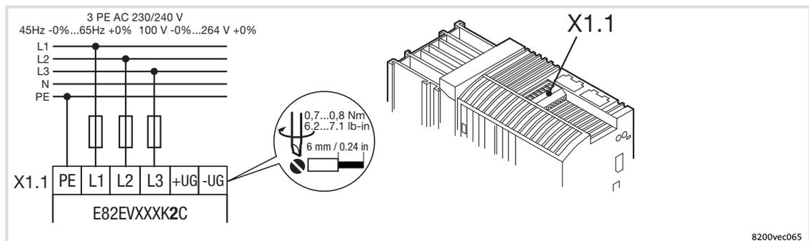
Fig. 6-13 Mains connection 230/240 V 3 ... 7.5 kW
