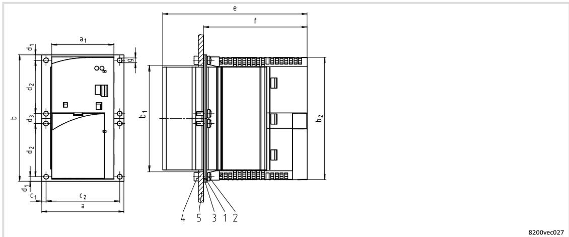
Fig. 5-2 Dimensions for thermally separated mounting 0.25 ... 0.75 kW
