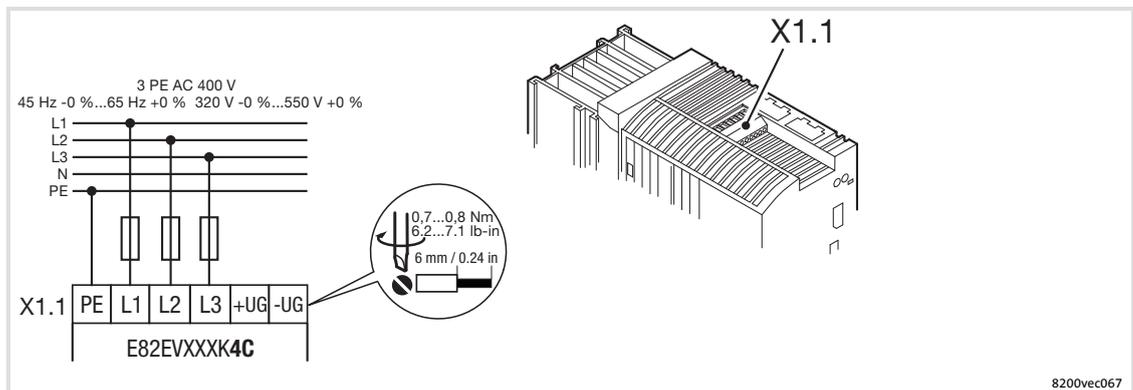
Fig. 6-14 Mains connection 400/500 V controller 3 ... 11 kW
