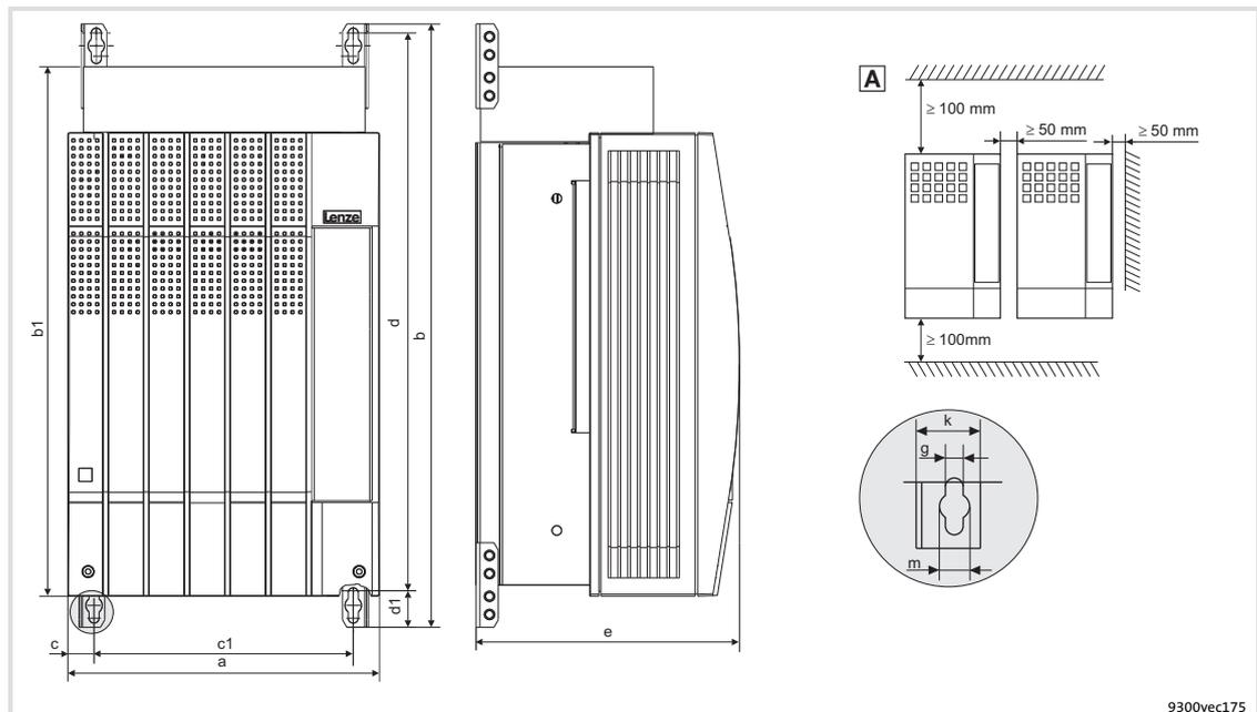
Fig. 5-23 Standard mounting with fixing brackets 55 kW
