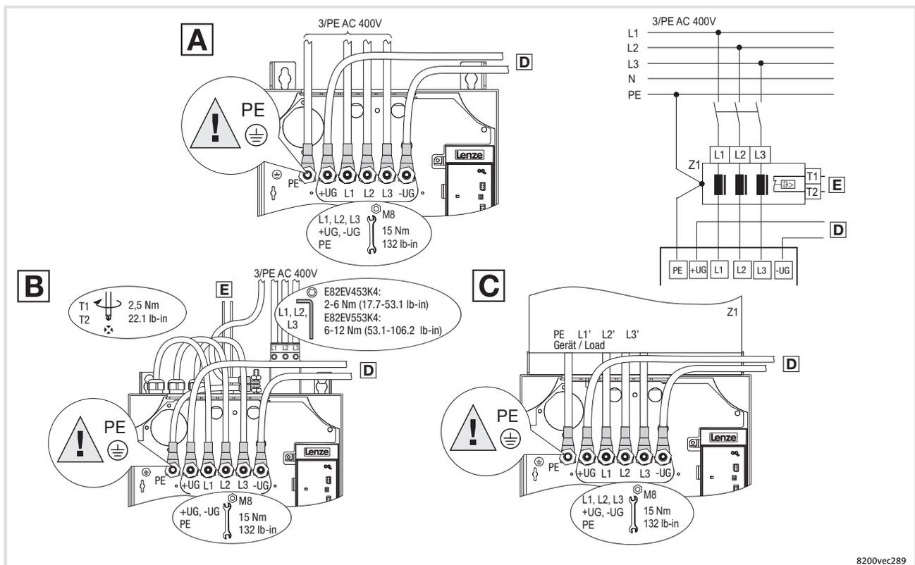
Fig. 6-22 Mains connection 45 ... 55 kW
