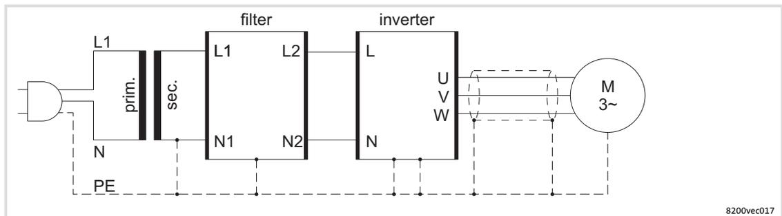
Fig. 6-1 Installation of a two-winding transformer (isolating transformer)
