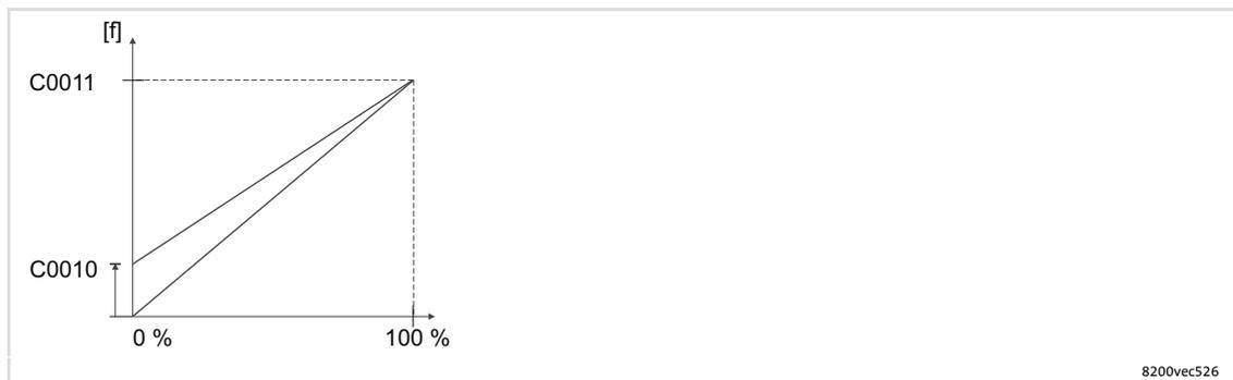
Fig. 10-5 Relation between setpoint and minimum and maximum output frequency
