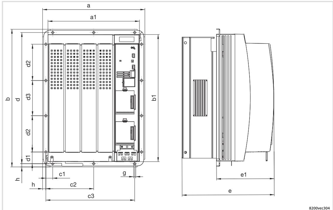
Fig. 5-18 Dimensions for thermally separated mounting 15 ... 30 kW
